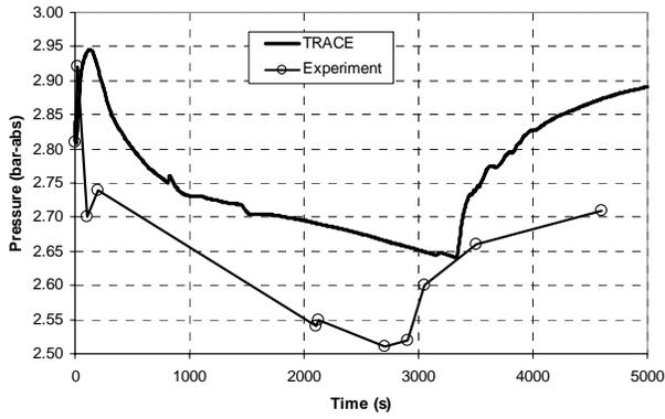
Figure 8: ISP-42 Phase B – Pressure in RPV
