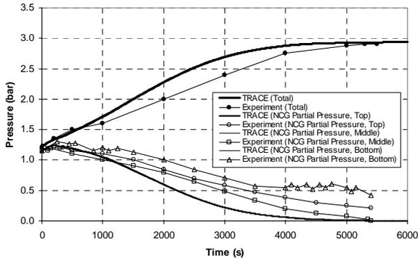
Figure 4: ISP-42 Phase A – Pressure in Drywell 1
