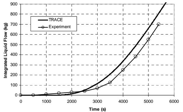
Figure 6: ISP-42 Phase A – Integrated Condensate Drain Flow from All PCCS Divisions
