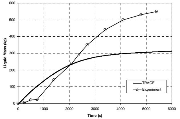
Figure 5: ISP-42 Phase A – Integrated Condensation in Drywell 1
