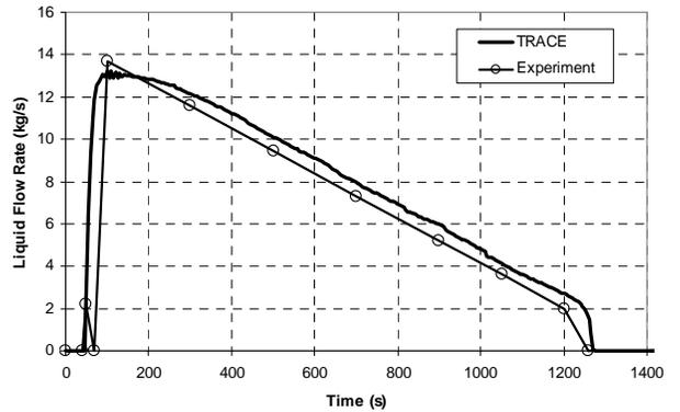
Figure 7: ISP-42 Phase B – Injection Rate from GDCS to RPV
