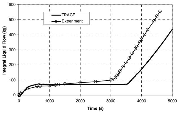
Figure 9: ISP-42 Phase B – Integrated Condensate Drain Flow from All PCCS Divisions
